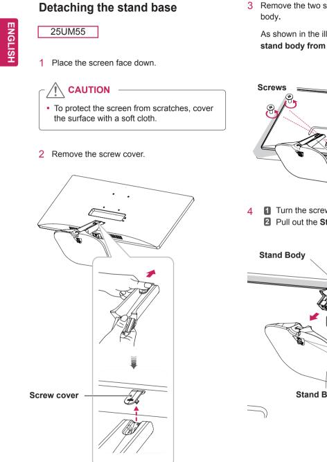
3 Remove the two screws on the back of stand
